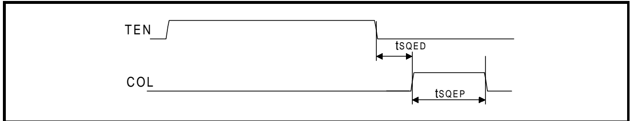
Figure 19: Mode 1 COL/SQE Output Timing/CI Output Timing
