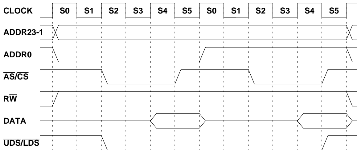
Figure 2-4. Word Read with 3-Clock 8-Bit Accesses
